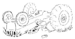
His tractor overturned in less than a second and crushed him to death. During 1994-99, 76 Kentucky farmers died in tractor overturns and 32 more died when they fell off tractors. ROPS and seat belts could have saved all 108 lives.
