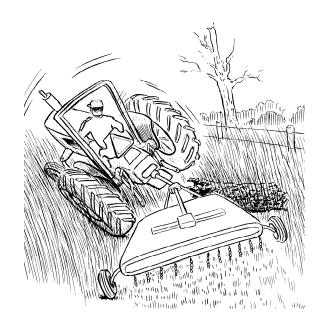
During a rollover, a ROPS and seat belt can be the difference
