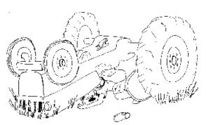
The tractor overturned in less than a second and he was crushed under its weight. In a recent six-year period, 76 Kentucky farmers died in tractor overturns. ROPS and seat belts could have saved all 76 lives.
