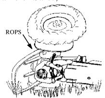
and within the "frame of safety" during an overturn.
