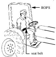
A fastened seat belt holds the driver on the seat
