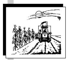
the key before attempting to clear the machine. The main drive shaft or cylinder should be turned with tools designed for that purpose. Hands should be clear of the combine's mechanism while the drives are turning. Once the plug has been cleared, remove all tools and replace shields before starting the combine.
