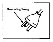
does not have a ground wire, then consider rewiring the device to accommodate the grounding feature. Another option is to use double insulated tools. These tools have an air space around the device to help insulate you from an electrical shock.
