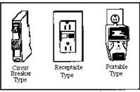
Another protective device that can be used is called a Ground Fault Circuit Interrupter, commonly referred to as a
