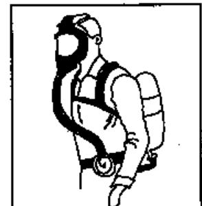
A self-contained breathing apparatus can be used where ever the user must work, such as in silos, manure pits, grain storage and fumigation of structures.
