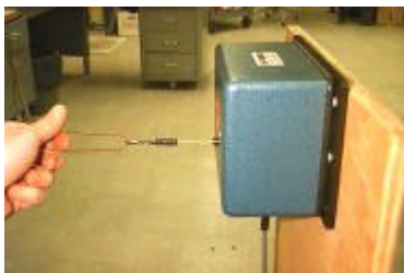
500 inch position/velocity transducer showing spring tensioned cable.
