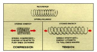
Springs are commonly used to help lift equipment, as shock absorbers, and to keep belts tight. **Springs may harbour potentially dangerous stored energy.** Always exercise caution when servicing springs.
