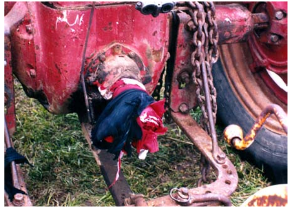
Figure 1. Clothing entangled on bolt on PTO tractor stub shaft
