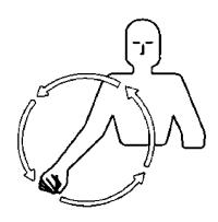
Start The Engine. Move Arm In A Circle At Waist Level, As Though You Were Cranking An Engine.
