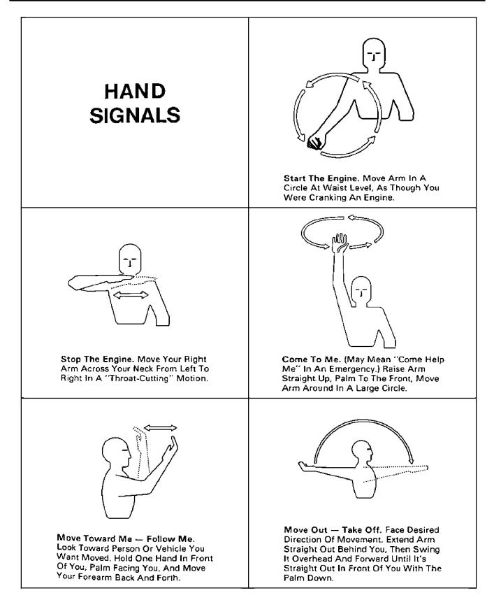
Hand Signals for Communicating with Machinery Operators (Part 1).
