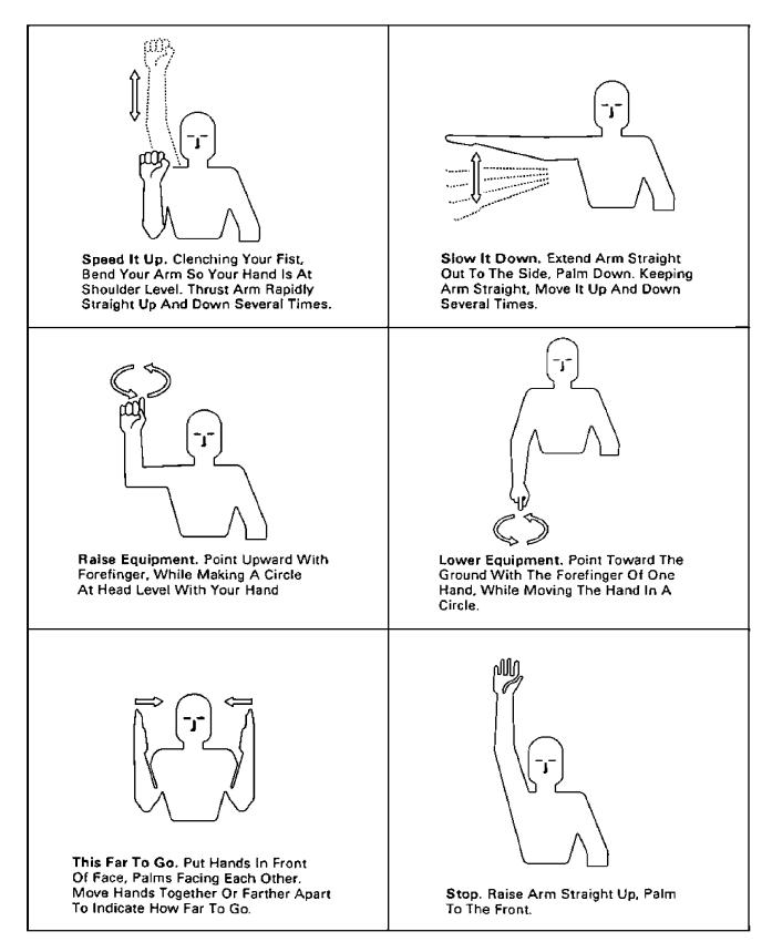
Hand Signals for Communicating with Machinery Operators (Part 2).
