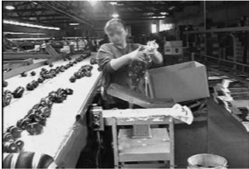
Figure 10 Manual Bag Packer Twist-Tying a Bag
