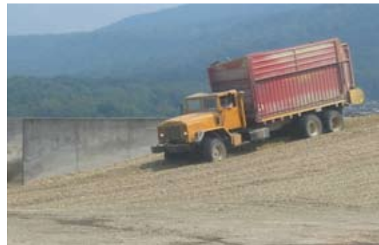
Figure 5. Bunker silo showing progressive wedge and dump truck operation.
