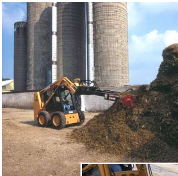
Figure 7. A defacer attachment on a skid steer or material handler boom helps break up silage over the entire face of the horizontal silo for safe removal of the silage.
