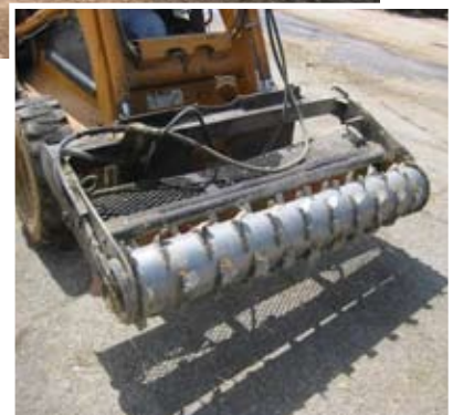
Figure 8. The exposed blades of a silage defacer pose serious entanglement and cutting hazards.
