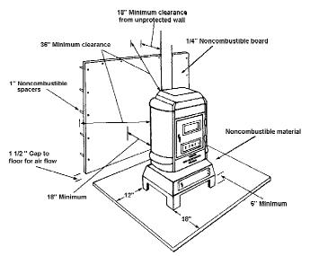
Figure 1. Reduced clearance installation (use wall and floor protection).
