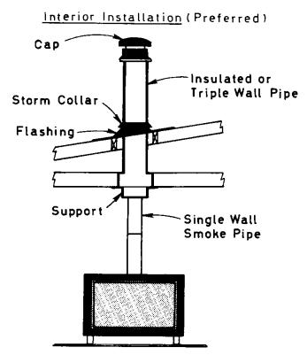
Figure 3. Metal chimney installation.
