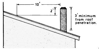
Figure 4. Proper height of a chimney.
