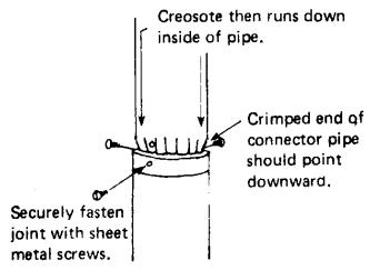
Figure 2. Proper connection of stovepipe.
