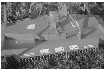
Running into a fixed object can shatter the blade and throw jagged chunks of metal out the discharge chute or under the housing. Obstacles such as ditches, rocks, and stumps can throw you off the tractor or cause a tractor upset. Be especially alert when objects may be hidden by tall grass, weeds or brush.
