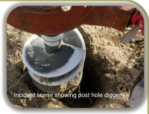
got caught in the unguarded, rotating PTO shaft of the post hole digger, causing his arm to become entangled and severed. He died at the scene. An investigation determined that the manufacturer requires a guard to be used and that individuals stay back 10 feet while the auger is being operated.
