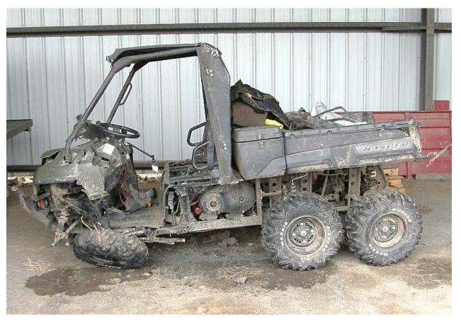
UTV after the incident showing the damaged left front that was struck by the pickup truck.
