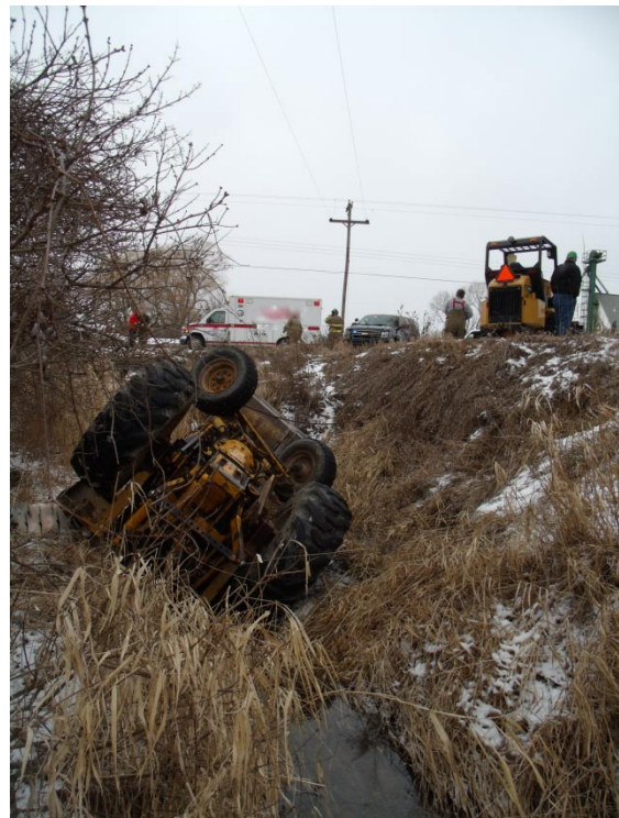
Figure 4. Final resting position of tractor. Note embankment slope.
