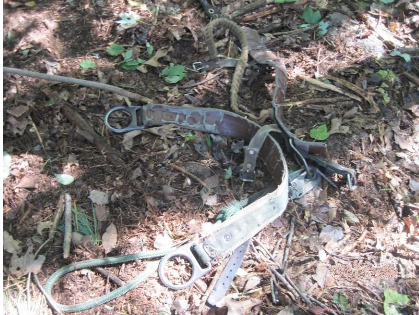
Figure 2 – Climbing gear that was in poor condition.
