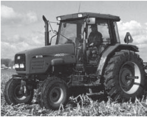
Figure 2. A ROPS with enclosed cab gives the operator the most protection from common hazards of tractor operation.
