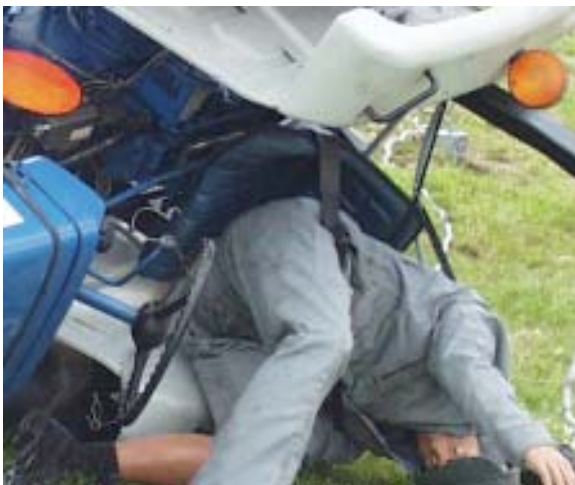
Figure 1. A buckled seat belt keeps the operator within the zone of protection of the ROPS during an overturn.
