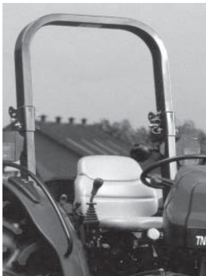
Figure 3. A foldable two-post ROPS allows tractor operation in low clearance situations without completely removing the ROPS.
