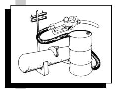
building could explode and spread the fire. Mount a tank elevated for gravity discharge on sturdy supports placed on a firm, level surface. Keep the area clear of weeds and trash to reduce fire risk. Remind machinery operators to stay away from the support structure and to not bump it when pulling up to refuel.
