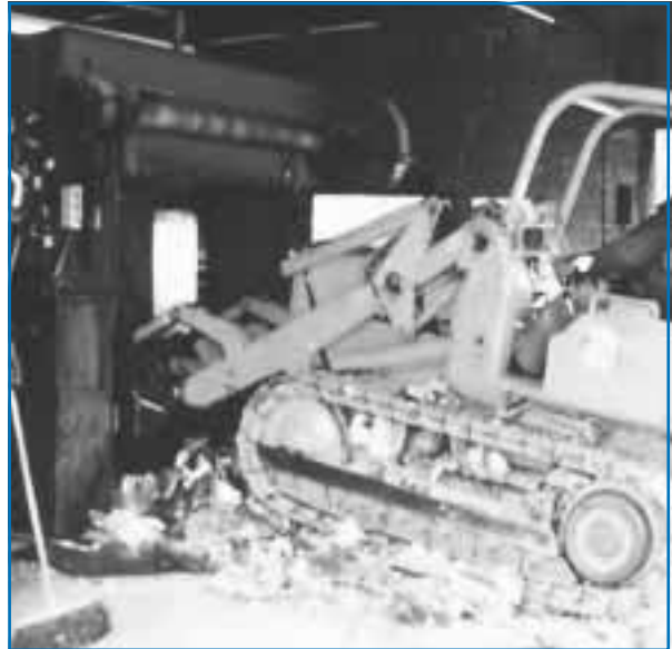
Figure 6. Vertical upstroke pit baler.
