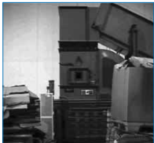
Figure 4. Automatic conveyor-fed baler.
