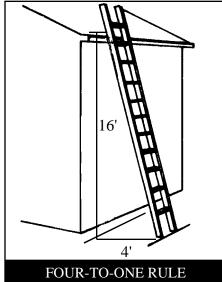
For every four feet of rise the base of the ladder should be one foot away from the object that the top of the ladder is resting.
