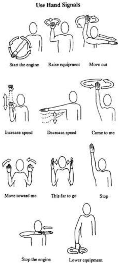
**Figure 1. Equipment is noisy; use hand signals to communicate between operator and other personnel.**
