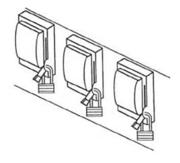
ing out and tagging power at its source is important while repairing or adjusting machinery because it ensures that power does not reach the machinery. For example, locking out the power to the augers in grain bins whenever they must be entered.
