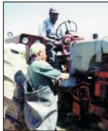
Correct jump start: Driver seated, with foot on brake.
