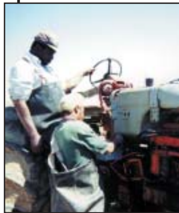
Incorrect jump start: Driver not in seat.
