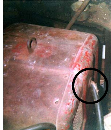
Figure 3. Damaged insulation on electrical cord
