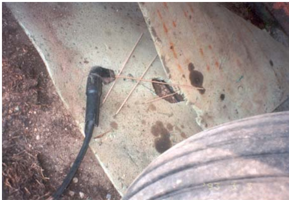
Figure 6. Stinger on mat, unused welding rods
