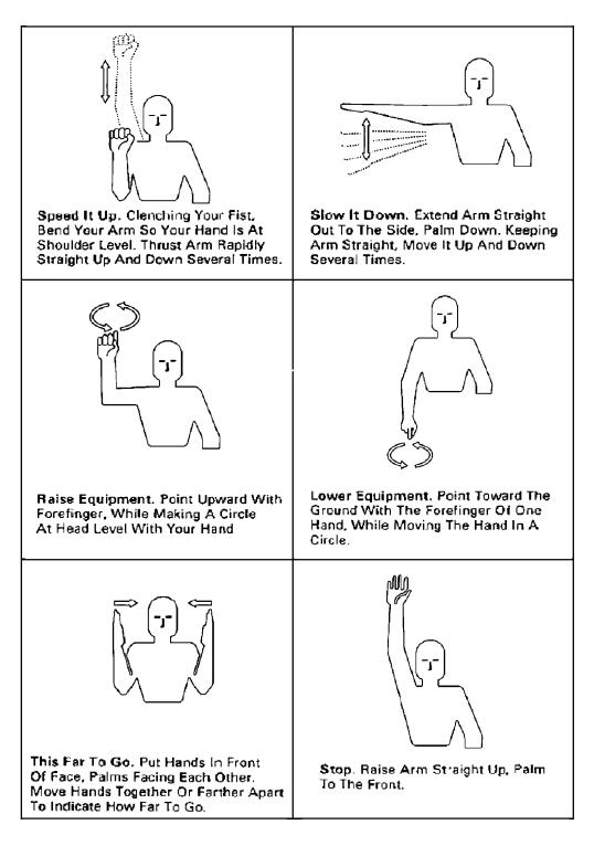
Hand Signals for Communicating with Machinery Operators (part 2; ASAE S351).
