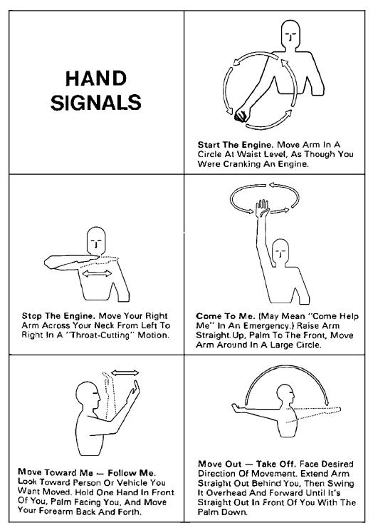
Hand Signals for Communicating with Machinery Operators (part 1; ASAE S351).
