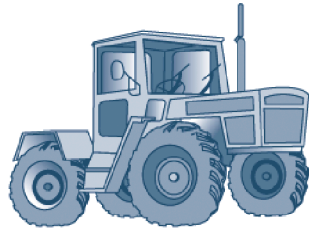
Enclosed cab (cab frame serves as ROPS)
