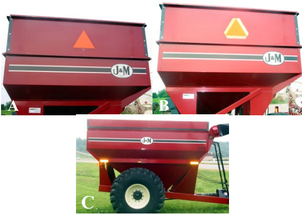
Photo 1: A properly placed SMV emblem that is clean, bright, and not obstructed. (A) SMV emblem shown during the day. (B) SMV emblem when illuminated with low beam headlights. (C) reflectivity of extremity markings.
