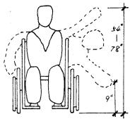
The average reaching distance of a seated adult: side reach maximum height overhead is 54 inches and the low side reach is 9 inches above the floor (Figure 2). This does not include reaching over an obstacle such as a counter. The maximum forward reach is 48 inches above the floor, also not over an obstacle.
