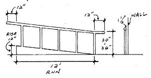
Landings are required at both the top and bottom of a ramp and should be at least as wide as the ramp (36 inches). Landings should have a 60-inch minimum length of clear space at both the top and bottom.
