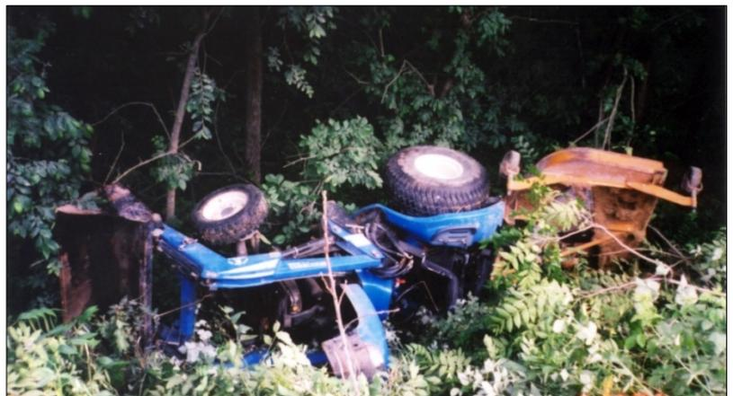
Scene involving a tractor overturn fatality where retractable ROPS was secured in folded-down position.
