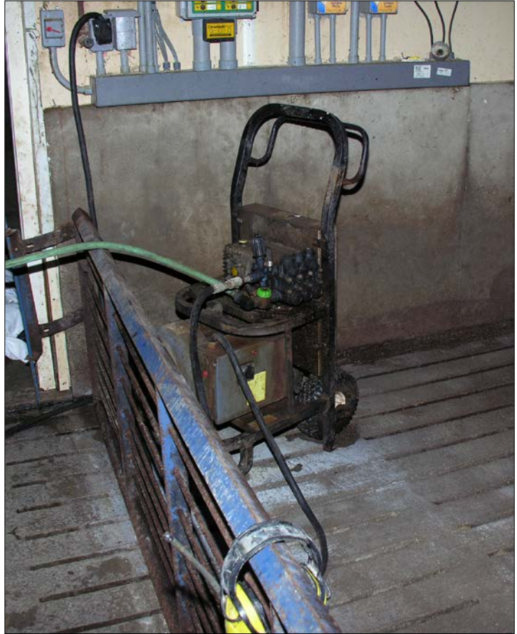
B. Pressure washer plugged into wall receptacle at site
