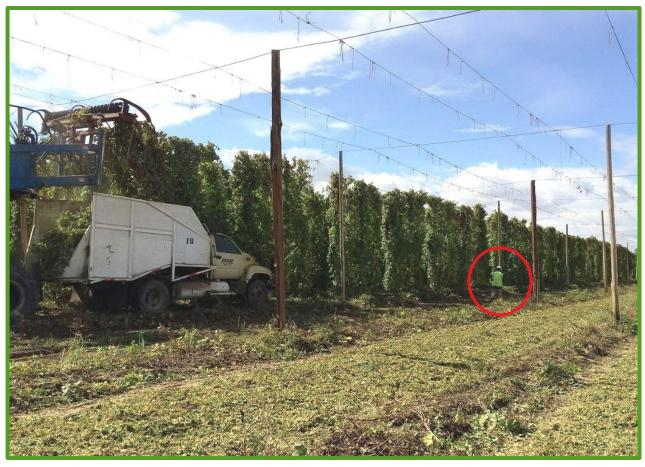
Top-cutter hop harvester cutting hop vines and dropping them onto a truck at the employer's hop farm. The field crew side tender is walking ahead and well clear of the top-cutter and truck, where he can be seen by the operators. He is wearing a hard hat and high-visibility safety vest.
