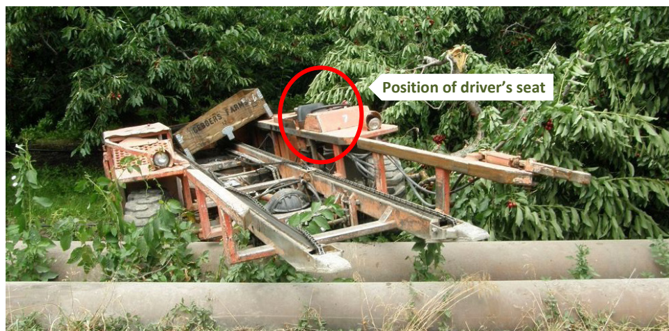
Incident scene showing the fruit bin carrier the laborer was operating on a cherry orchard road when it rolled backwards downhill, causing him to be thrown from it and severely injured.
