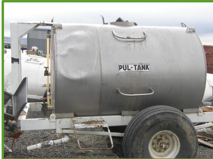
1,000-gallon capacity trailer-mounted water tank that was being towed by the tractor.
