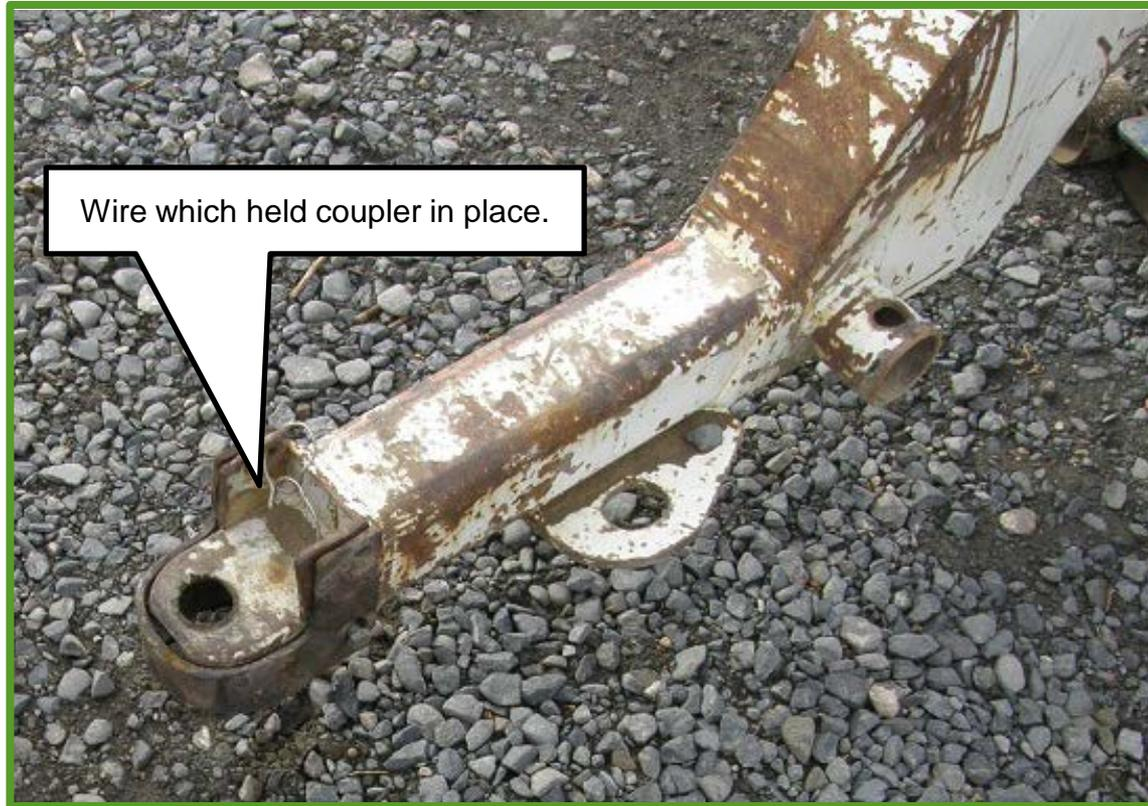
Coupler and water tank trailer tongue after the incident. A piece of wire was used to replace the missing locking bolt.
