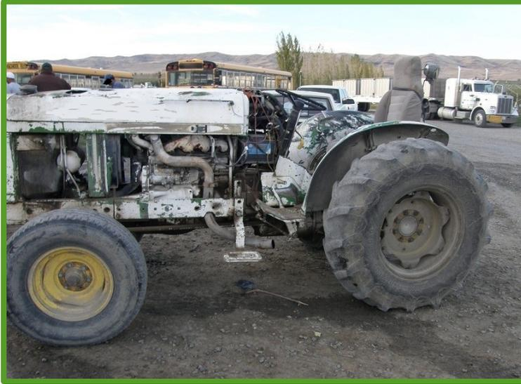
Tractor involved in the incident. It did not have a rollover protective structure (ROPS) or a seatbelt.
