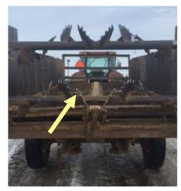
Photo of straw spreader bars. Arrow indicates where worker's clothing was entangled in rotating beater bar.
