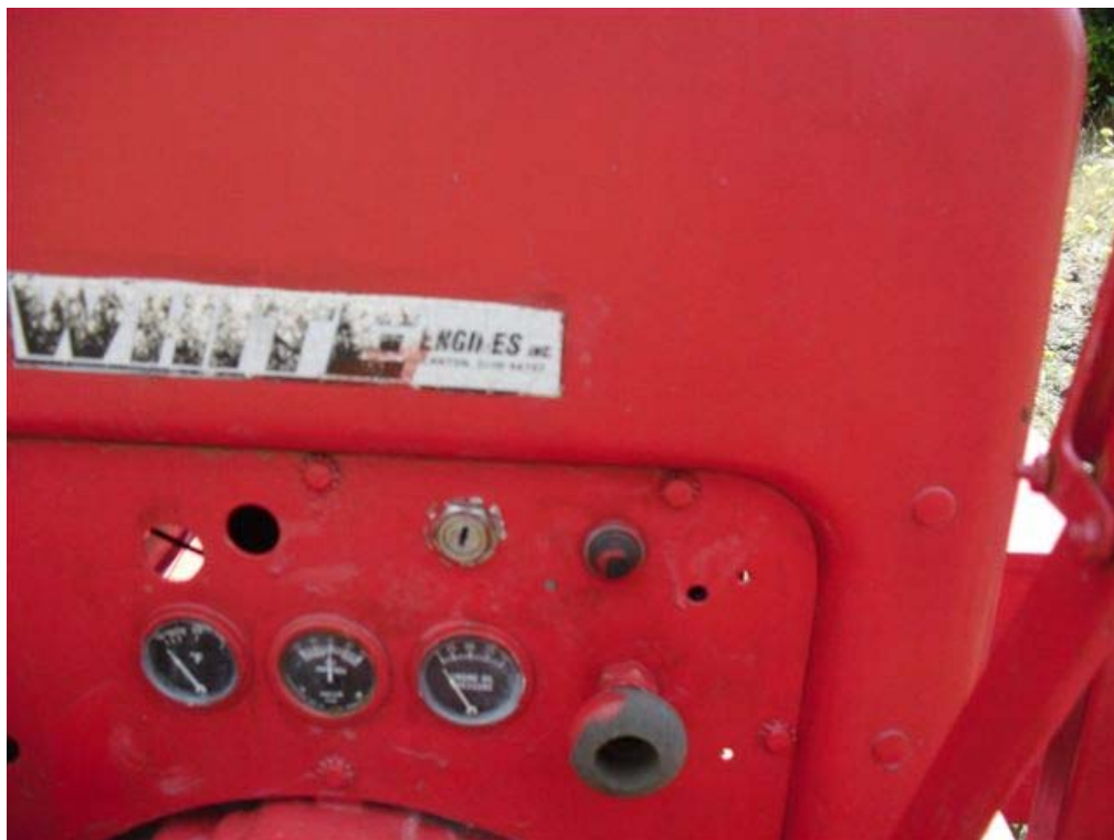
Exhibit 8. The control panel on the wood chipper.
