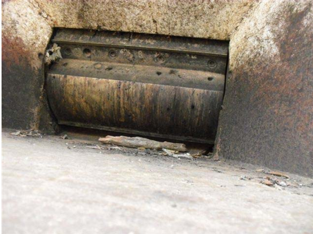
Exhibit 7. The blades attached to the rotating drum that chip brush.
