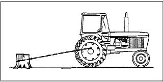
**Figure 7.** An example of unsafe hitching. The "angle of pull" does not lower of the front end rises, increasing the risk of a rear overturn.
