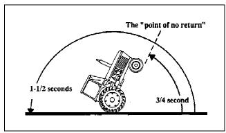
**Figure 3.** The "point of no return" during a rear turnover may be reached in 3/4 of a second. (Source: Agricultural Safety, Deere and Company, Inc.).
