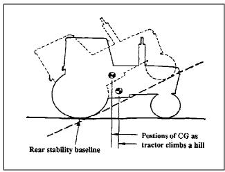
**Figure 4.** The center of gravity moves toward the tractor's rear stability baseline when the tractor is headed up a hill, or if rear wheels are below normal ground surface, such as when stuck in soft ground.
