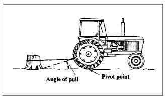
**Figure 5.** The "angle of pull" is rearward and downward. The point at which the rear tires contact the ground becomes the pivot point.
