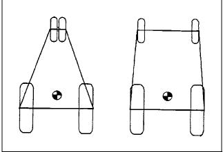
**Figure 1.** The stability baselines of a tricycle and a wide front-end tractor, respectively.
