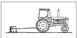
**Figure 6.** An example of safe hitching. The drawbar will lower if the front end rises. This reduces the "angle of pull" and the risk of a rear overturn.
