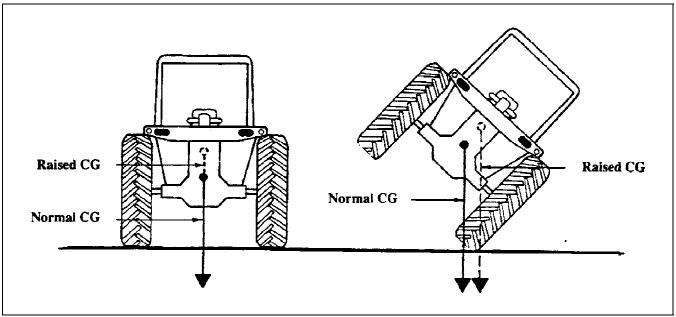
Figure 2. A higher center of gravity allows a side overturn to occur more quickly.
