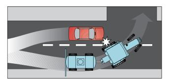
Why it happens: Like semi-truck drivers, operators of large farm vehicles, such as combines or tractor-wagon combinations, sometimes make wide left turns. Farm operators may swing to the right before making a left turn because they need the extra room to line up with a farm gate or driveway. This can be confusing, especially if you think the farm operator is moving over to let you pass.
